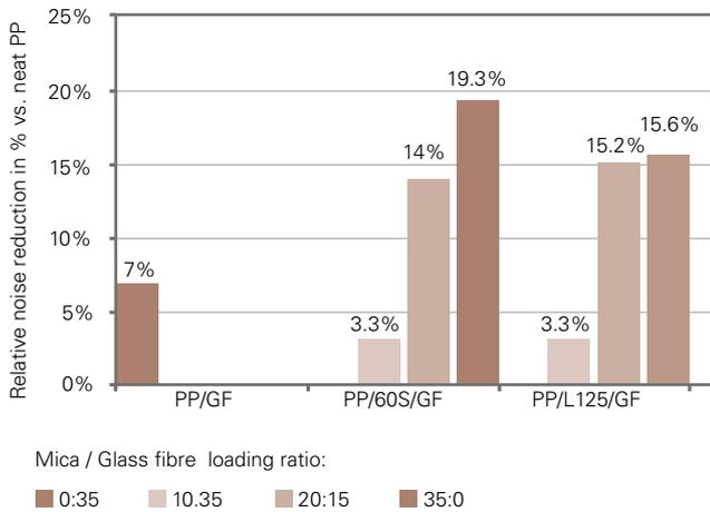
Figure 9. Relative noise reduction vs. neat PA 6.6
